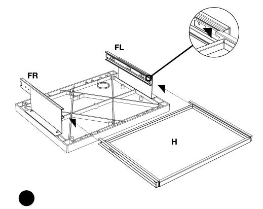
Collect parts: **H**. Align the pullout shelf **H** runner so that the runner snaps into place into the **FL** & **FR** brackets. Pull the shelf out to make sure it is fully seated. Tighten screws **A**. Pullout keyboard shelf assembly is now complete.
